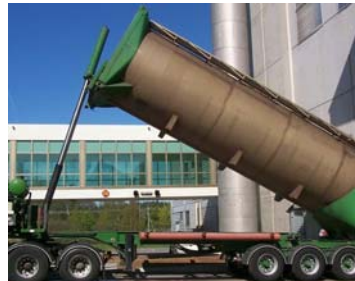
Emptying silo vehicles
